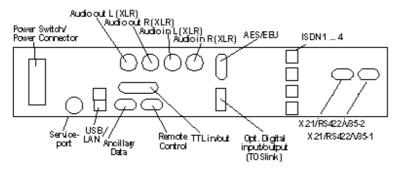
The plugs for the X.21 connection does not conform to standards. Instead of the usual 15 contacts in two rows (SubD), the socket plugs on the rear of the CENTAURI II 3000/3001 has 26 contacts in three rows (HD). The socket plugs can thus be used either as V.35 or X.21 connection. A corresponding cable with the necessary pin configuration can be obtained from Mayah.
