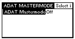
This dialog allows you to activate or deactivate the ADAT Mastermode. **Turned off**, the Centauri II can be clocked via the ADAT input interface (optical TOS Link interface).
