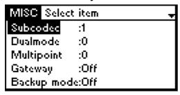
enables to configure the gateway feature of the Centauri. Gateway functionality means that Centauri routs received audio from one interface to another one (e.g. MPEGL2 audio received at ISDN is sent out as MPEGL3 audio via IP).
