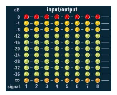
Through the levelmeter, you will receive notice about the signal strength of the incoming, but also of the outgoing signal. The level of the levelmeter can be configured via "SETUP / FRONTPANEL / LEVELMETER".
