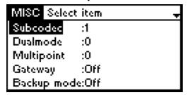
enables to configure the backup feature of the Centauri. Backup means that Centauri establishs automatically another connection if framing is lost.
