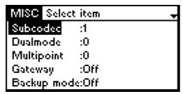
Although CENTAURI II can be used as two individual Mono (sub)codecs only one user interface is available. This setting lets the user select which codec (either 1 or 2) the input and display apply to.
