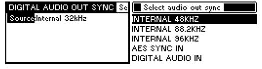
defines the AES/EBU output clock source. If any of the 'internal' sources is selected, the AES/EBU Sample rate is also affected.
