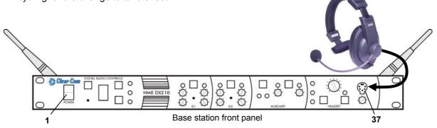
If a local headset will be used, plug it into the HEADSET connector (#37) on the front panel of the base station.
