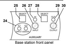
If the auxiliary equipment requires two-way communication, have someone listening at the auxiliary unit. Press the AUX IN/OUT SELECT button (#28) until both the IN and OUT lights (#s 27 and 29) go on. While speaking into your headset microphone, adjust the **OUT** control (#30) above the light to the desired listening level at the auxiliary unit. Listen to the audio input in your headset as you adjust the **INPUT** control (#26) below the light to the desired level.
