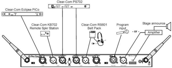
Typical equipment connections to the rear panel of the base station
