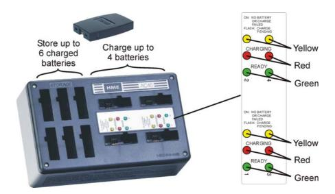
NOTE: Batteries should not be left in charge ports after being fully charged. If a battery is left in a charge port for more than three weeks, the yellow indicator may light up. In this case, it does not indicate a faulty battery.
