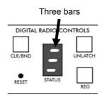
Secondary base station operating in primary mode when no primary base station is found
